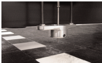
Fabric Drill - up to 9.5 mm (3/8 in) diameter
