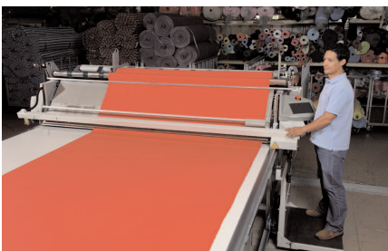
GERBERSpreader™ tension-free material spreading system
