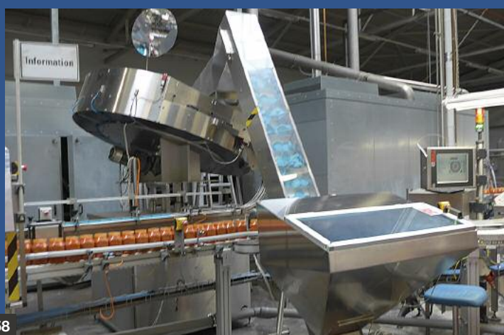
"SIEM" CAP 06 PP (2006) - Deckelaufschraubmaschine • capping machine, with cap elevator
