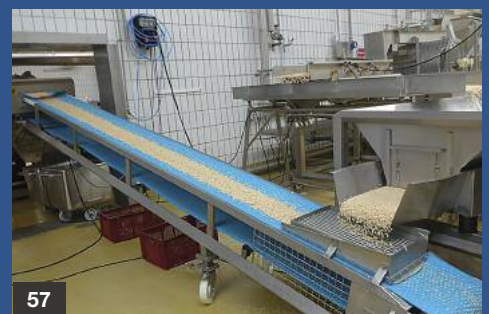
63 “THERMO RAMSEY” (2010) Kontrollwaage • check weigher 65 “GRONEMEYER” - Förderer/Synchronverteiler • conveyor synchron distributor 95 “GRONEMEYER” - Flaschen-Vert.-Förderanlage • bottle vert. conveyor 90 “JORGENSEN” - Flaschen-Depalettierer • bottle depalletiser 57 “FLEXLINK” - Schrägförderband • inclined conveyor, with metal detector
