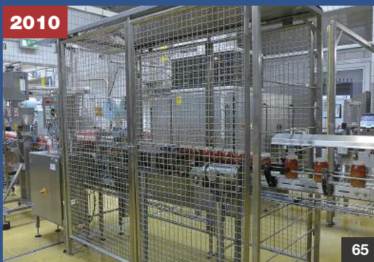
63 “THERMO RAMSEY” (2010) Kontrollwaage • check weigher 65 “GRONEMEYER” - Förderer/Synchronverteiler • conveyor synchron distributor 95 “GRONEMEYER” - Flaschen-Vert.-Förderanlage • bottle vert. conveyor 90 “JORGENSEN” - Flaschen-Depalettierer • bottle depalletiser 57 “FLEXLINK” - Schrägförderband • inclined conveyor, with metal detector
