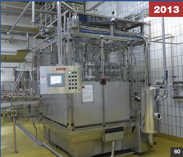
“ZACMI” 0288 (2013) Rundläufer-Kolbenfüller • rotary piston filler with 28 turning valves, filling volume up to max. 1250 ml
