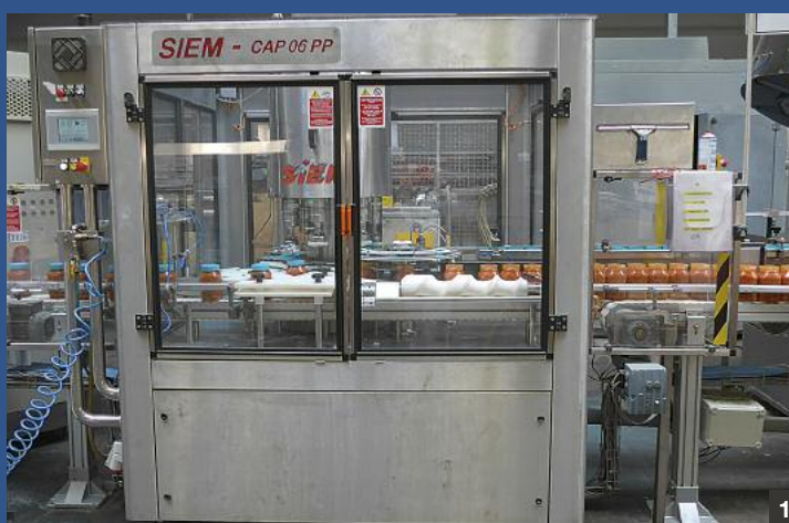
"SIEM" CAP 06 PP (2006) - Deckelaufschraubmaschine • capping machine, with cap elevator
