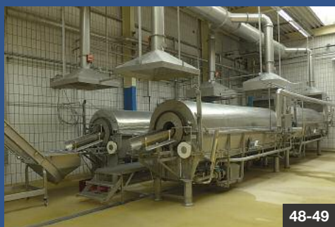
“STEINER” TW 653/1000 - Trommel- waschmaschine • drum washing machine
