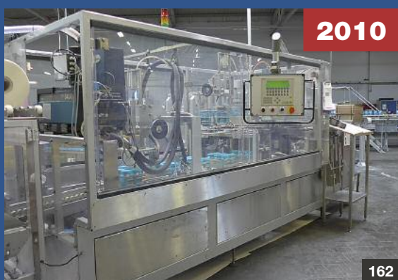
"SIEM" CAP 06 PP (2006) - Deckelaufschraubmaschine • capping machine, with cap elevator
