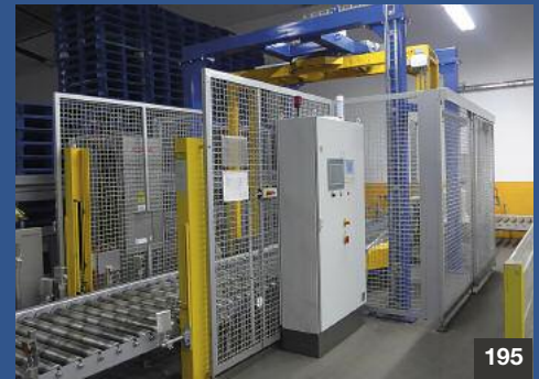
Palettenstretchwickler • pallet stretch wrapper
