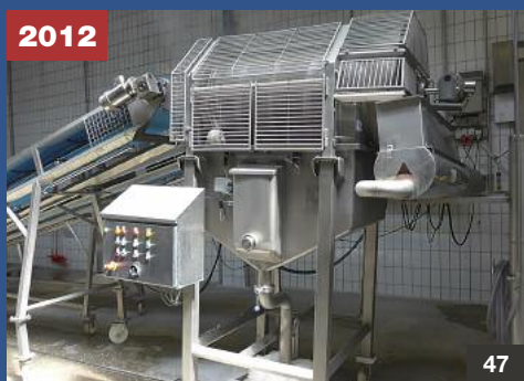
“STEINER” TW 653/1000 - Trommel- waschmaschine • drum washing machine
