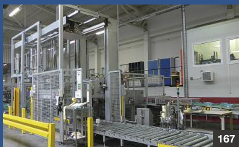
"MEYPACK" - Palettierer • palletizer pallet size 1000 x 1200 mm
