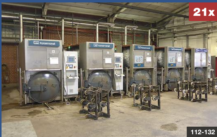
112- "STOCK"/"ATMOS" 132 (general overhauled 2013-2008) 21 Autoclaven • 21 autoclaves, for 4 cage trolleys, temp. max. 165/200 °C
