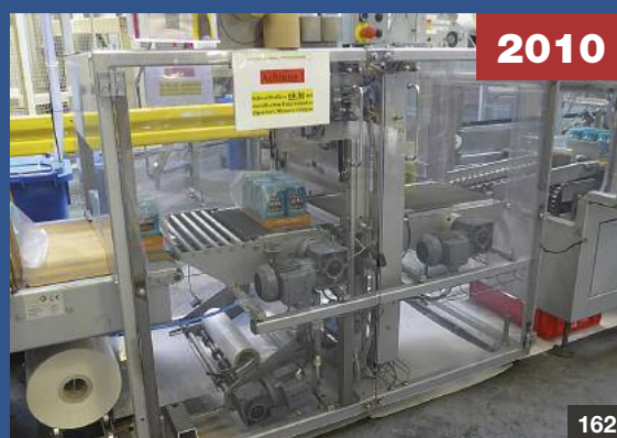
"SIEM" CAP 06 PP (2006) - Deckelaufschraubmaschine • capping machine, with cap elevator
